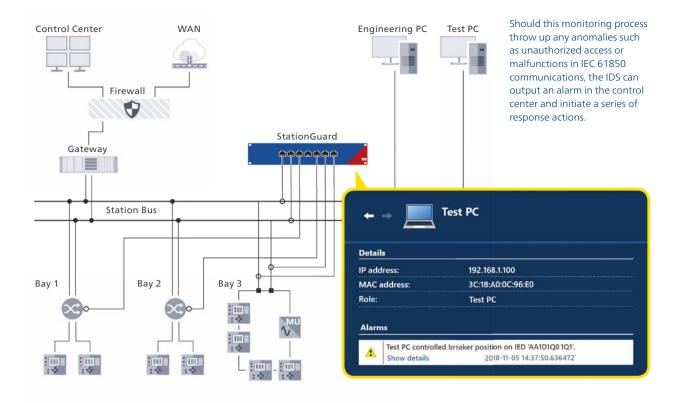
The process and support networks are logically and physically separated. Communications using the IEC 61850 Ed. 2 protocol are implemented on a different interface from that used to access devices for engineering or maintenance purposes. The entire process network is segmented, with each segment being separated from the others by a redundant firewall.
