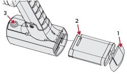
E Open the lid (1) of the battery housing, and insert the battery connectors first and then the charge gauge (2) facing upwards. Ensure the battery is all the way inside the housing. Close the lid.
