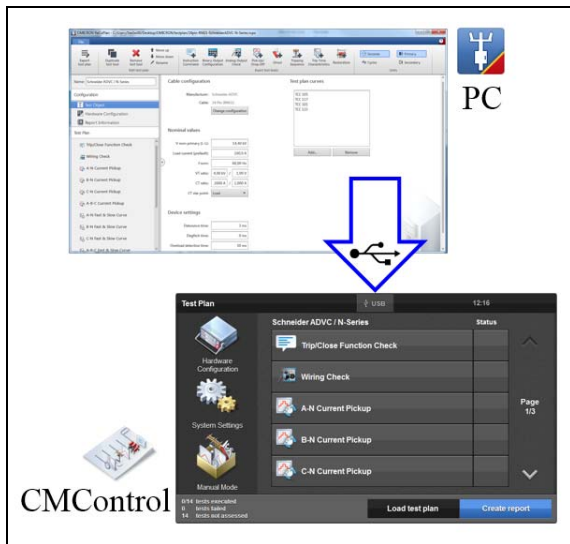
Fig. 6 Test plans created on PC and loaded from PC to the controller CMControl
