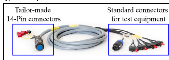
Fig. 1 Typical 14 pin recloser testing interface
